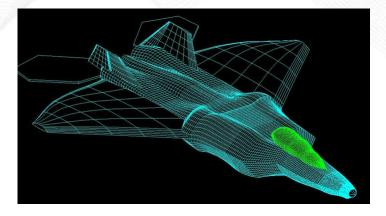
Lockheed Martin F-22 Raptor, 1996, new materials like titanium and composites make up 80% of the structure by weight
