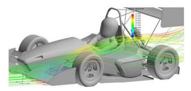
Optimization of aerodynamics for a Formula 1 race car using a CFD (Computational Fluid Dynamics) model
