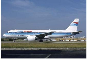
Airbus A320, 1988 – first civil aircraft with digital fly-by-wire flight control
