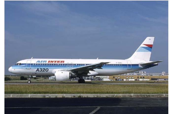
Airbus A320, 1988 – first civil aircraft with digital fly-by-wire flight control
